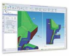
The calculation and display of **drafts and undercuts** are extremely quick, even on very big parts. WorkXPlore 3D automatically colors drafts and undercuts according to the mold stripping axis. Precise draft angle values are displayed dynamically as the mouse is dragged over the surfaces and can be inserted by default in the 3D model.
